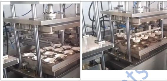
Above photograph shows bowls cured in a compression moulding press being taken out
