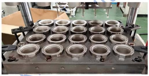
Above photograph shows lower platen of a compression moulding press with moulds for cups. The mixed material blanks of predetermined weight are placed in the mould cavities and the press is closed and material is cured with heat and pressure to form rigid finished product (in this case cups)
