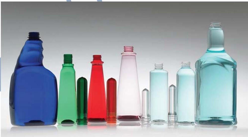
These are manufactured by Injection moulding of Preforms and then Stretch Blow moulding of these into bottles and containers.
